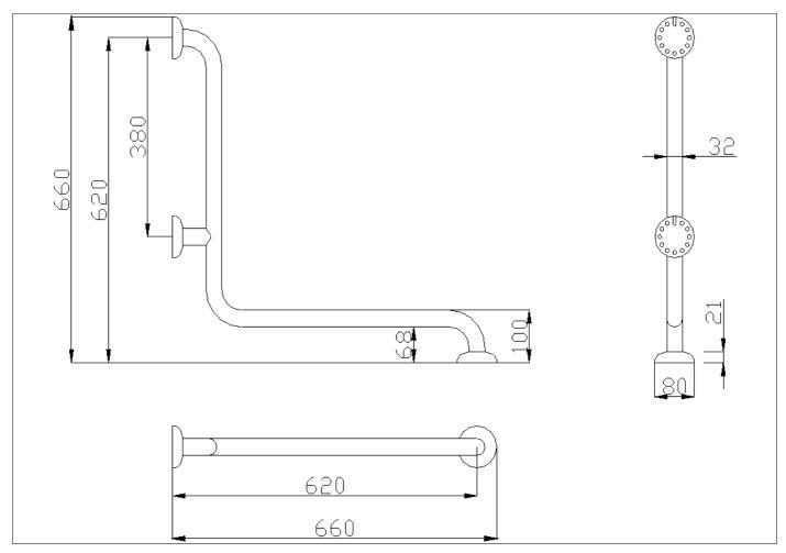
Corner grab bar made of stainless steel AISI 304 pipe, with polished finish
